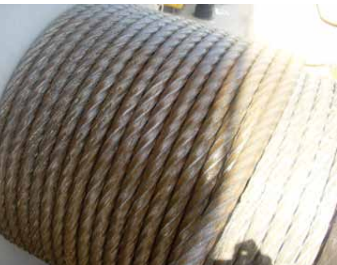
Wire rope that is properly treated on a regular basis with penetrating and coating lubricants will be protected from the elements and other negative factors and will provide a longer useful service life.
