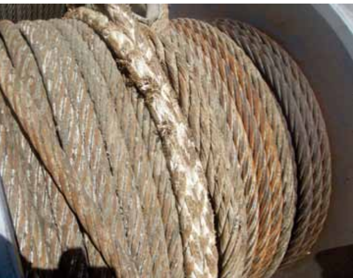
This spool of wire rope shows some of the damage that can occur due to a variety of factors, including worn sheaves, improper winding and splicing practices, improper storage, high stress loading, shock loading, corrosion, oxidation, and abrasive wear.
