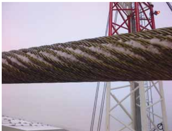
This 100-mm non-rotating wire rope used on an offshore crane is totally dry and covered in ice and snow prior to lubrication.
