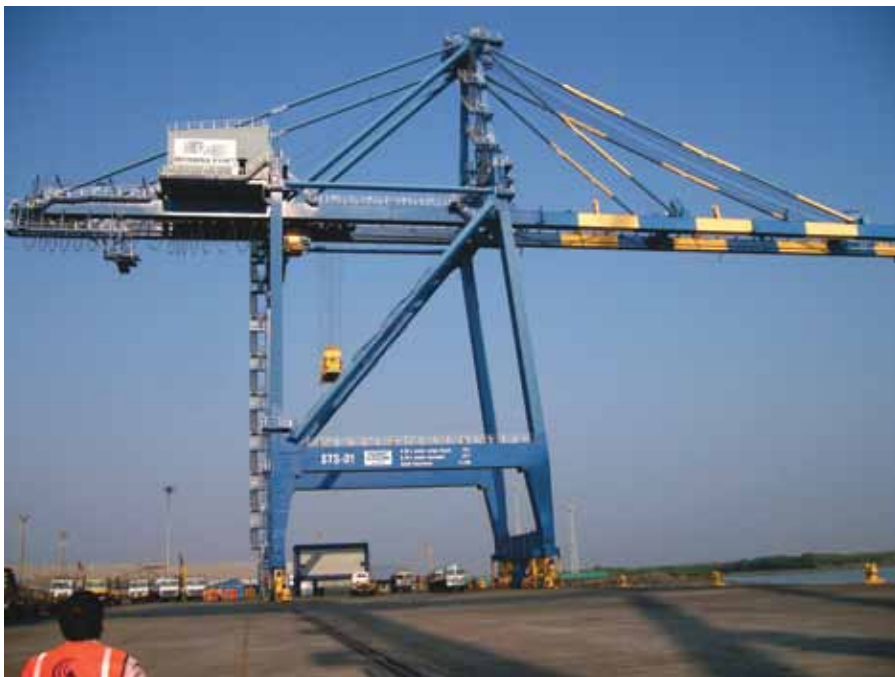
Large dockside cranes (also known as container cranes or ship-to-shore cranes) are used for loading and unloading containers from ships. Wire ropes are an essential part of the crane's operation, and they must withstand demanding environmental conditions. Without proper lubrication, they require frequent repair or replacement.
