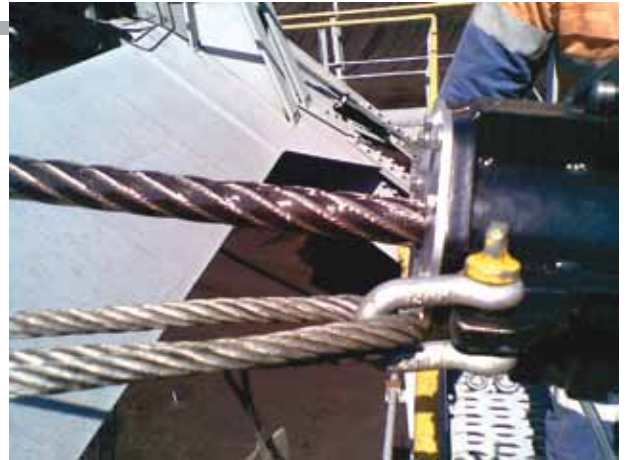
Freshly greased wire rope comes out of the back end of the Viper automatic lubricating unit.
